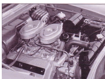
1958 Chrysler Fire Power 392 cid, 380 hp@5200 rpm, 435 lbs@3600 rpm (SAE)
