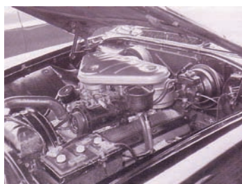
1955 Chrysler Fire Power 331 cid, 300 hp@5200 rpm, 345 lbs@3200 rpm (SAE)
